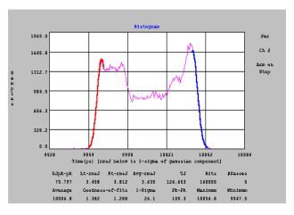
Figure 4 - Histogram tail search and fitting algorithm application for clock jitter, using Wavecrest's DTS system as the measurement instrument.
