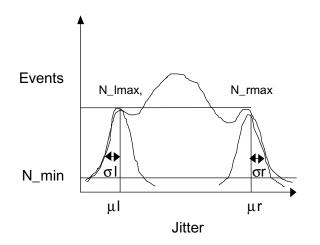
**Figure 1 -** Drawing of total jitter histogram in the presence of DJ and RJ.
